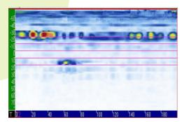
C-scan of weld displaying indications as high reflection signals (red and yellow amplitudes). The weld geometry is displayed in the C-Scan for localization. Cursors are available after the scan for determining the position of indications with respect to the weld geometry.
