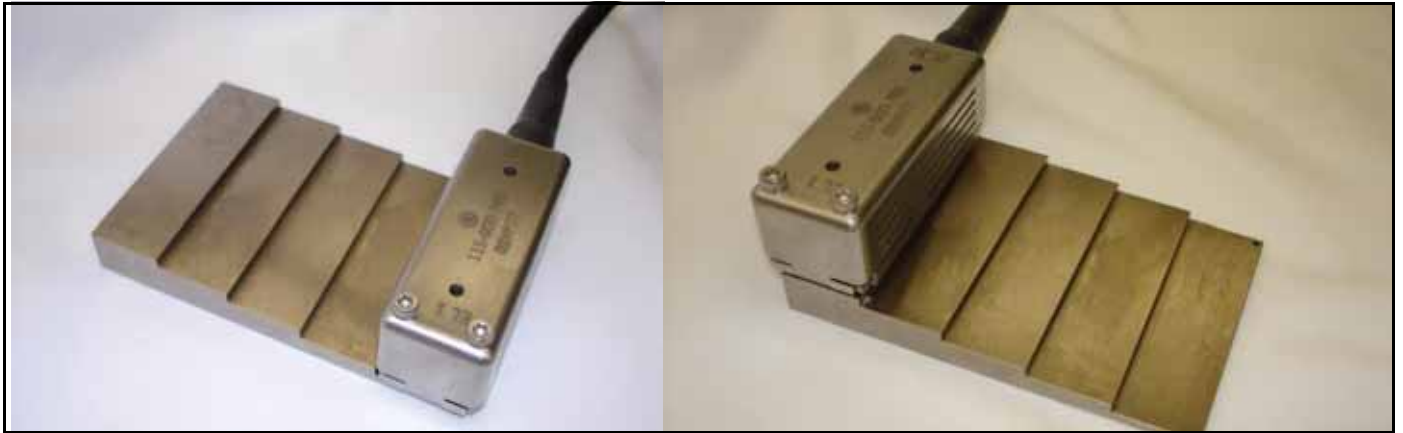
Figure 72: Calibration Probes on 0.1-inch block and 0.5-inch block
