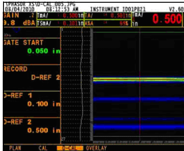
Figure 76: Adjusting the Gain for D-REF2 Standard
