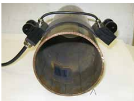
Eddy current surface and subsurface inspection for flaw detection in metals
