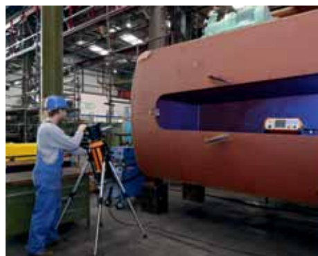
Inspection of ship assemblies using industrial X-ray
