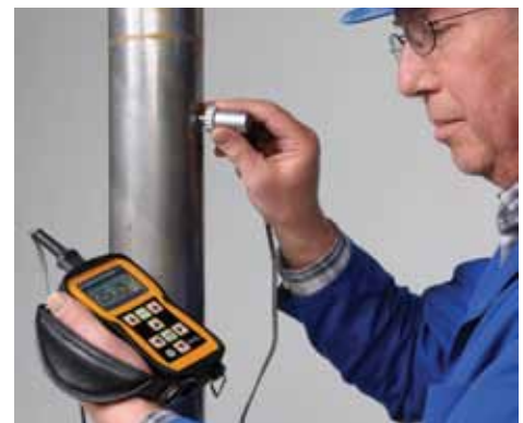
DM5E ultrasonic thickness gaging of pipes
