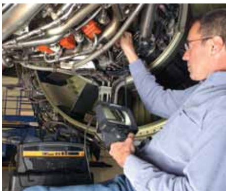
Aircraft engine inspection using the XLG3™ VideoProbe
