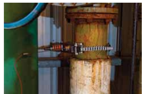
Rightrax™ permanently-installed sensor on oil & gas pipe section
