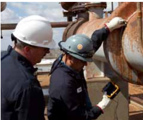
USM Go/DMS Go portable ultrasonic flaw detector and thickness gage in one
