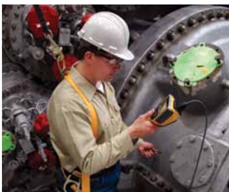
Large gas turbine inspection with the XL Go+ VideoProbe®
