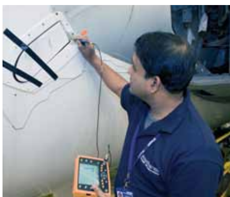
Aircraft inspection with the Phasec 3 series flow detectors
