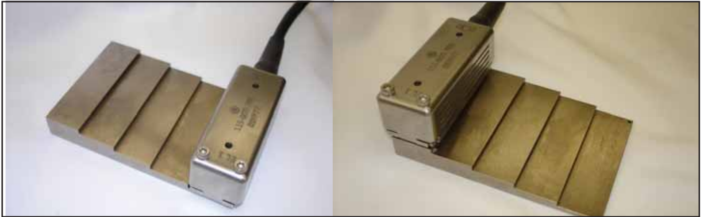
Figure 72: Calibration Probes on 0.1-inch block and 0.5-inch block
