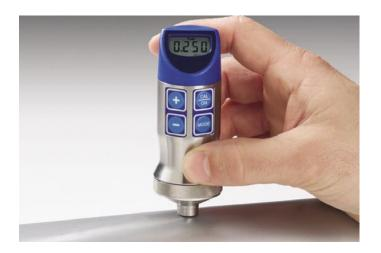
The PocketMIKE's integrated product design combines the instrument and transducer into a single package allowing for true single hand operation and providing a very capable yet simple to use device.
