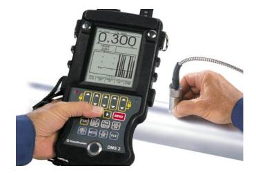
The DMS 2 is the right solution for demanding inspection problems dealing with corrosion inspection. The programmable data recorder can be configured from the PC and has the ability to store masses of thickness data for downloading to a computer for storage and analysis.
