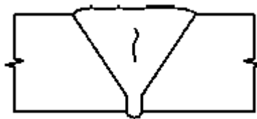
15 Centerline Crack, Single Vee (sub-surface) UT, RT
